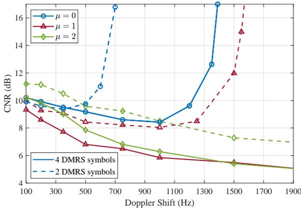
FIGURE 11. CNR (dB) against Doppler shift (Hz) for 5G New Radio in TU-6 mobile channel. Numerologies 0,1 and 2, MCS 3.
