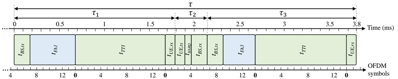
FIGURE 6. User plane latency for numerology 0, with slot based scheduling of 14 symbols (1 ms). Average frame alignment.
