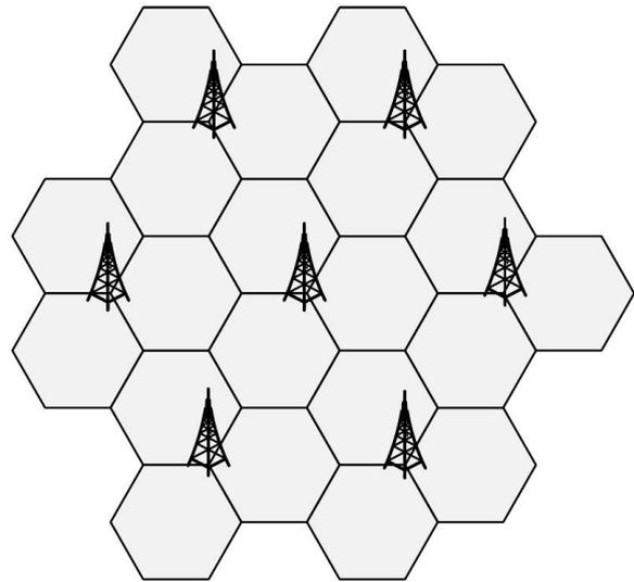
FIGURE 5. Hexagonal site layout for UMa and RMa [4].
