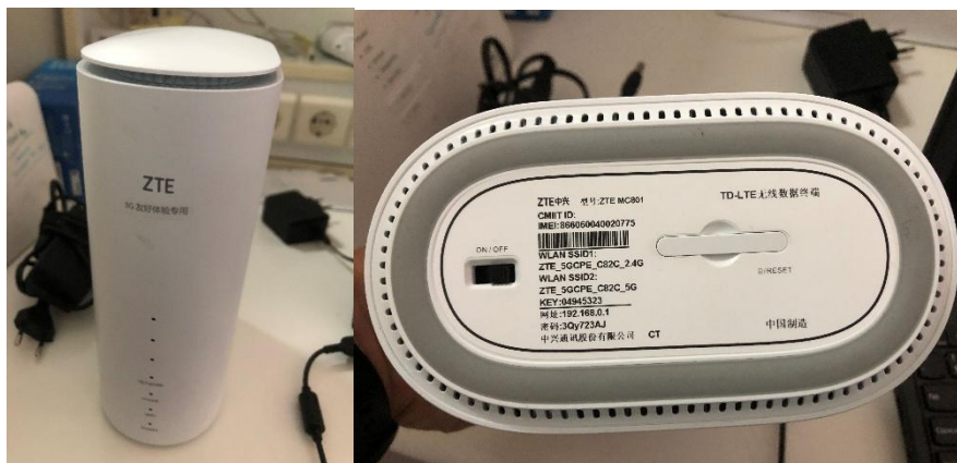
Figure 46. ZTE 5G-Router/modem model MC801 that supports the 3,5-3,8 GHz frequency band.
