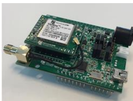
Figure 29. Development kit with mounted embedded modem.
