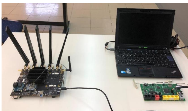
Figure 47. Oxygen Broadband 5G Router Prototype based on Quectel & Realtek Reference boards.
