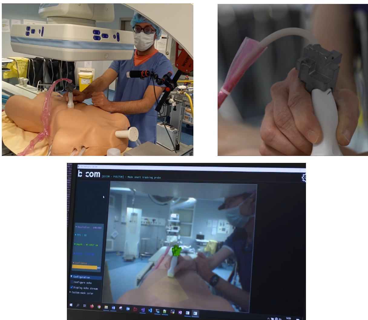
Figure 91. Probe with the 3D marker and the video of the camera to localize the probe in its environment
