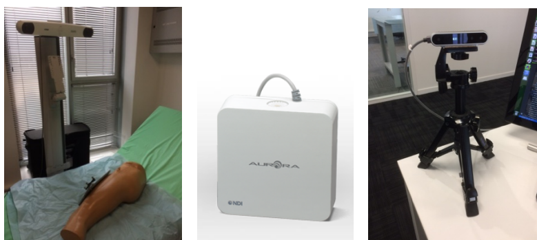
Figure 78. NDI Polaris, NDI Aurora and RGB-D camera.
