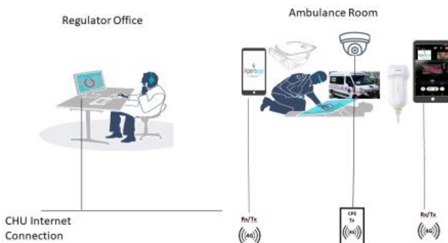
Figure 31. 2nd setup – 4G / 5G based user tests with Philips Lumify application screen shared in AMA XpertEye solution.
