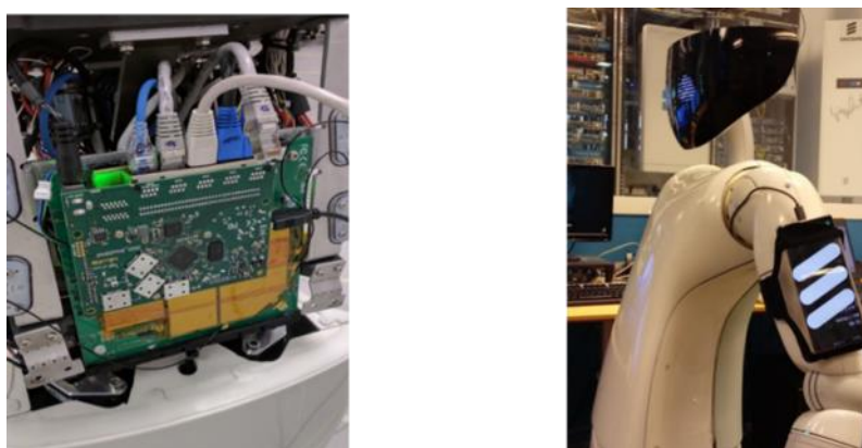
Figure 64. The Mikrotik router inside the robot and the 5G smartphone attached to the arm of the robot.
