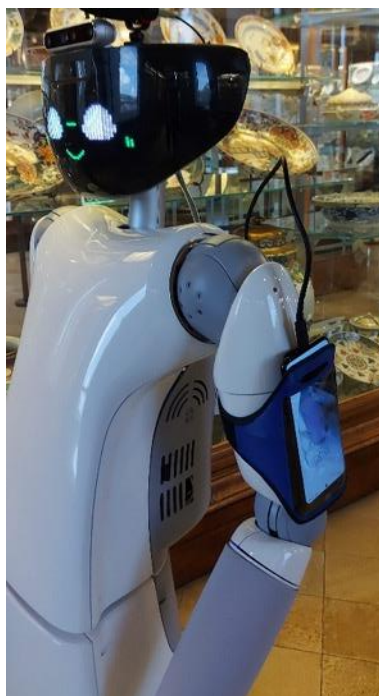
Figure 51. The 5G phone attached to the left arm of the R1 robot.
