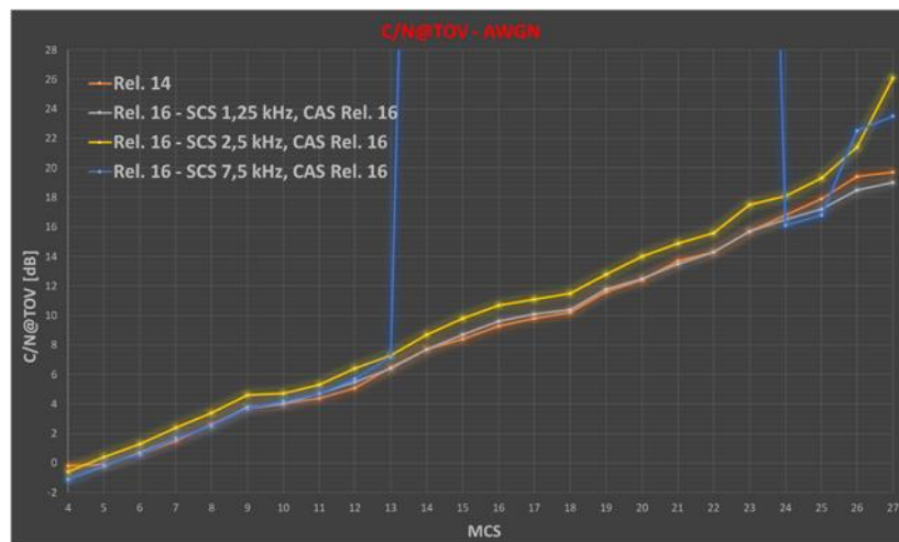
Figure 88. C/N@TOV with AWGN (Bw= 5 MHz, SCS= 1.25 kHz, 2.5 kHz, 7.5 kHz).
