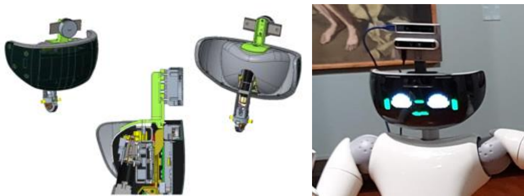
Figure 62. The head cover of the robot modified to mount the additional sensors for localization and mapping.
