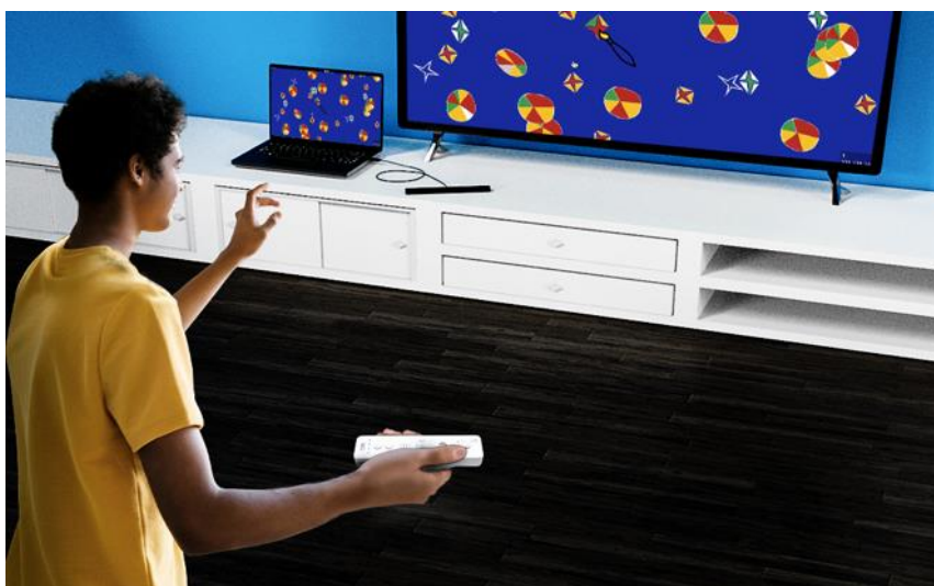
Figure 30. PC with WebHID API web application connected to the Display (TV-Set or Projector) and Wiimote player playing the UC1.b Interactive Wall at home (Flexible portability and scalability of the system).
