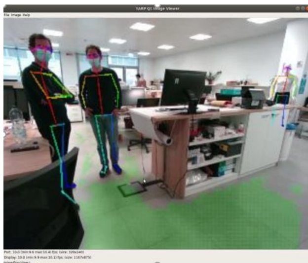
Figure 54. Additional video processing for human detection, during the robot teleoperation.
