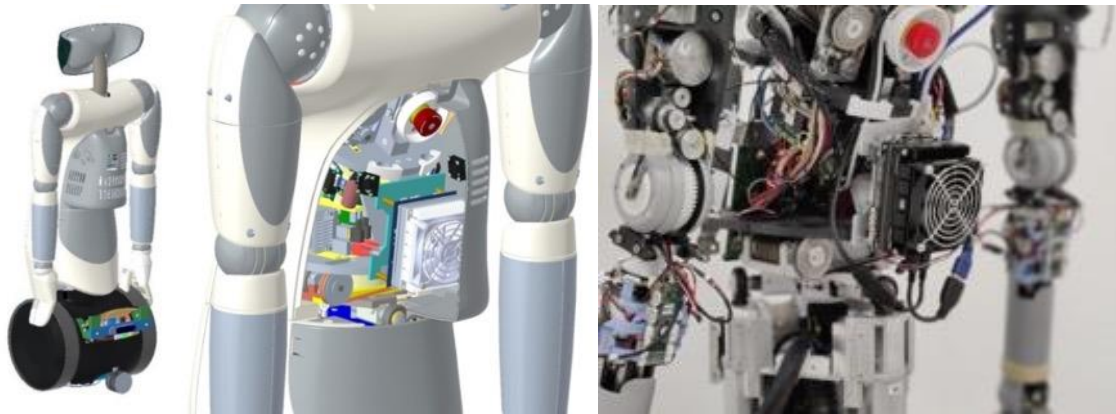
Figure 63. The back cover of the robot redesigned to host the additional Xavier AGX and the router.
